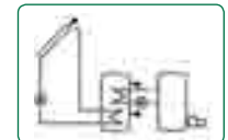
Solar system with 1 storage and thermostatic after-heating
