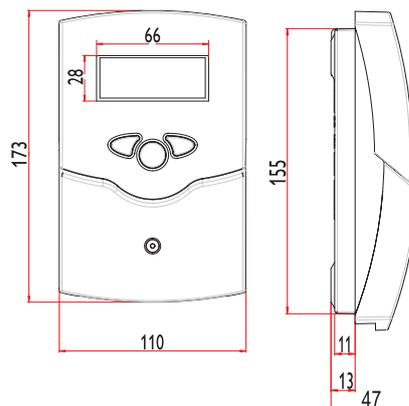
The DeltaSol® BS is a controller for standard solar thermal systems. It provides a clear operating concept and is equipped with a system-monitoring display. Flashing symbols for sensors, pumps and valves show temperatures, temperature differences and active actuators. The DeltaSol® BS controller is available in 4 versions
