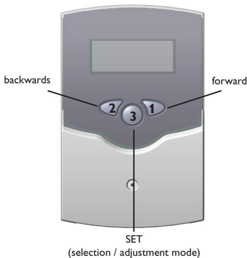
The controller is operated via the 3 push buttons below the display. The forward-button (1) is used for scrolling forward through the display menu or to increase the adjustment values. The backward-button (2) is similarly used for scrolling backwards and reducing values.
