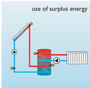
The thermostat function works independently from the solar operation and can be used for using surplus energy or for after-heating.
