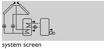
The system screen (active arrangement) shows the scheme which has been selected. The screen consists of several system component symbols, which are - depending on the current status of the system - either flashing, permanently shown or „hidden“.
