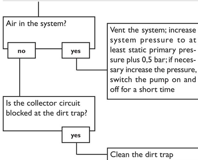
Pump starts for a short moment, switches-on/off again, etc.
