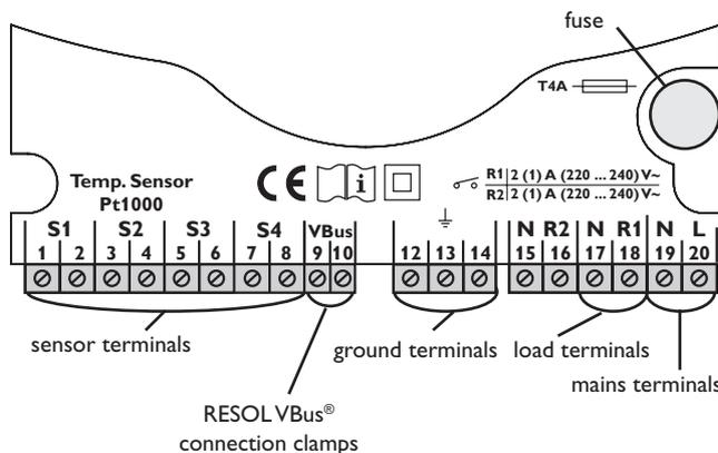
The power supply to the controller must be carried out via an external power switch (last step!) and the supply voltage must be 220 ... 240V~ (50 ... 60 Hz). Flexible cables must be attached to the housing with the enclosed strain relief and the corresponding screws.
