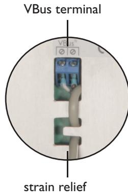
The Smart Display SD3 can be operated in parallel with a controller and additional modules via a bus line.
